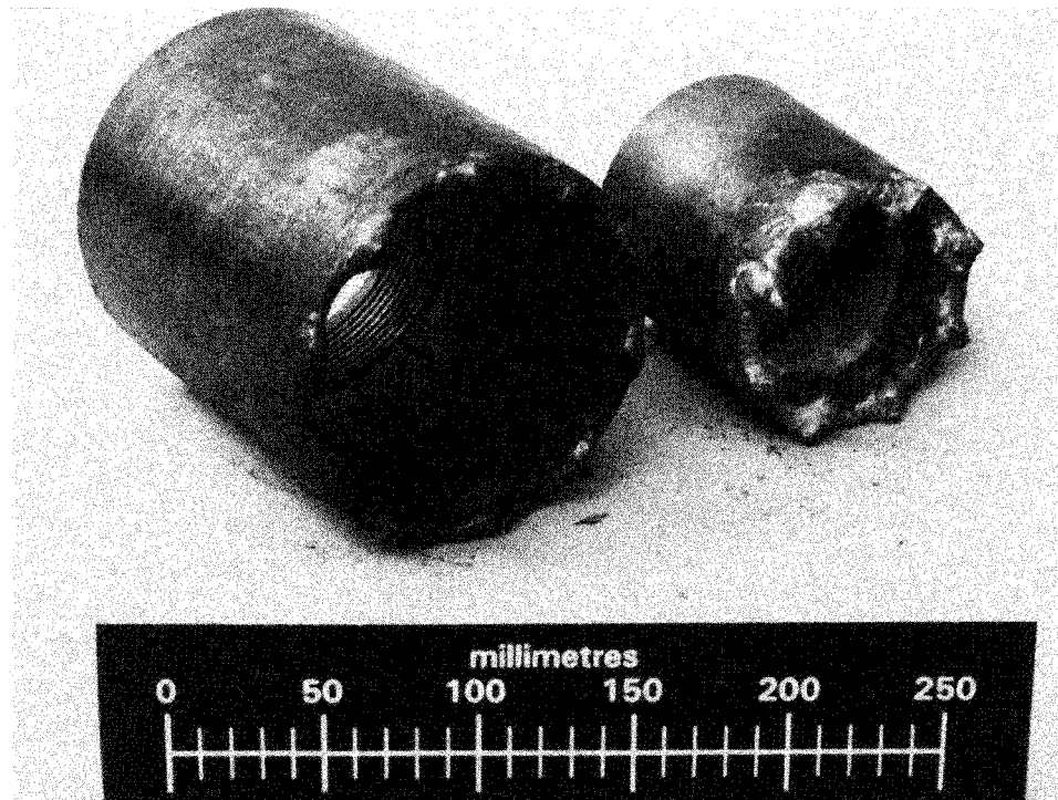
Figure 3-17. Photograph of a standard carbide insert bit and a pyramid carbide bit
