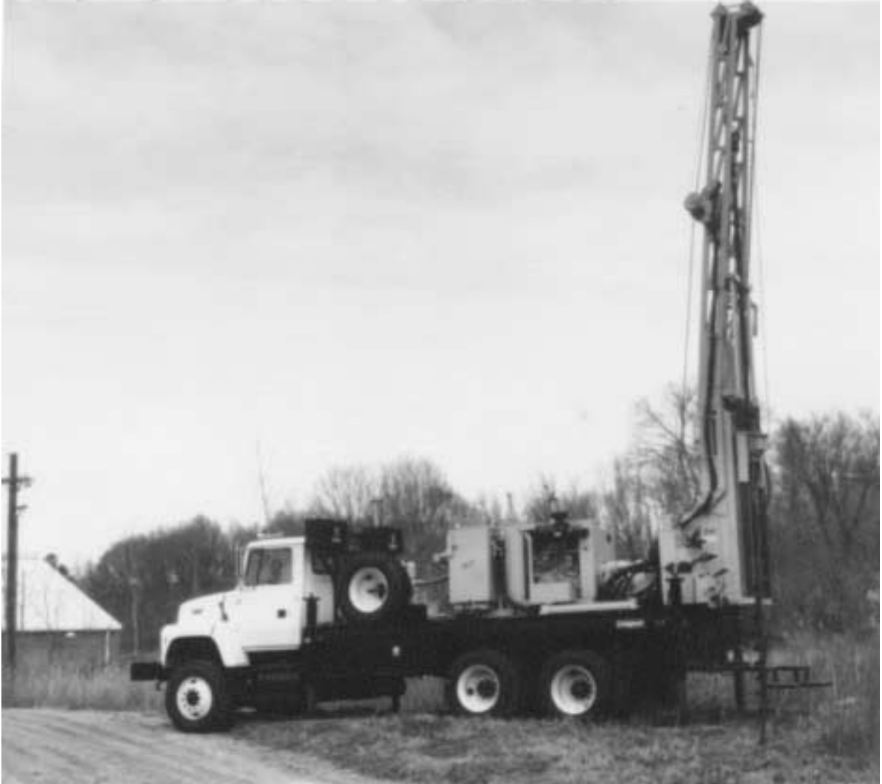
Figure 3-1. Truck-mounted rotary drill rig with a hydraulic drive system
